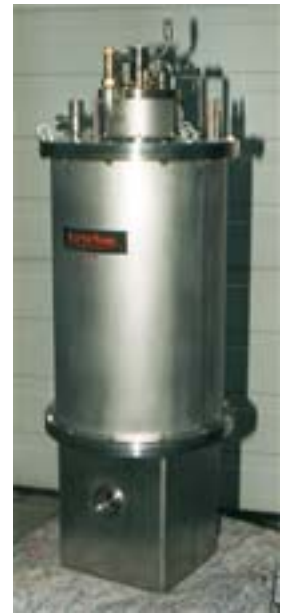
Bath-Cryostat-Magno-Spektro with continuous flow cryostat 7-T split coil magnet
